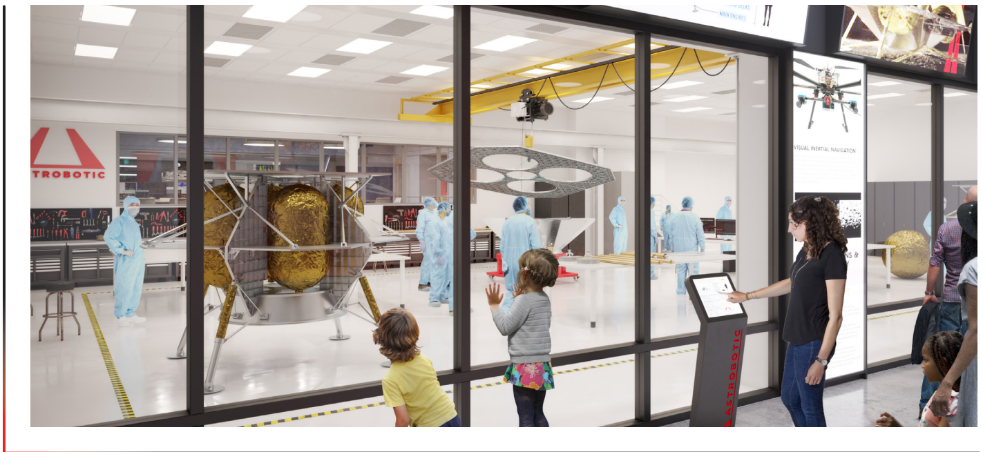
Astrobotic Headquarters and Integration Facility contains two ISO Class 8 cleanrooms for Integration.
