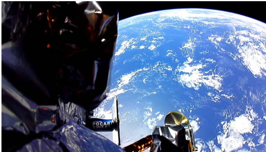
FIGURE 3: This image was taken by camera 1 moments after successful separation from United Launch Alliance's Vulcan rocket. Counterclockwise from top left center is the DHL MoonBox, Astroscale's Pocarí Sweat Lunar Dream Time Capsule, and a Peregrine landing leg. In the background is our big blue marble, our home planet, Earth.
